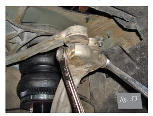
9. Loosely install the lower fork/shock mount bolt into the lower control arm bushing. Also, loosely reinstall the track link to chassis bolt as well as the sway bar end link (Figs. 34 & 35)
