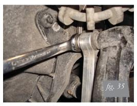
10. Make sure the lower fork/shock mount is fully seated against the shock adapter, install the nut and bolt and torque to 40 Nm + 180 degree turn (29.5 lb.-ft. + 180 degree turn) (Fig. 36).
