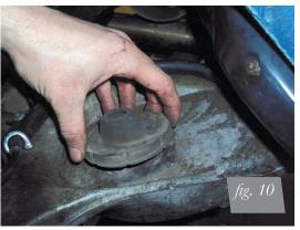
6. Directly above the upper coil spring perch, remove the rubber plug (figs. 11-12).
