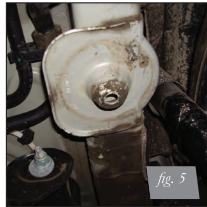
Previously Cut Spring Perch with Aftermarket Shock
