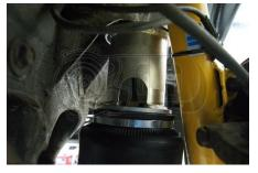
• Support the LCA and lift this up to meet the bottom of the air bag, now allowing you to fix the LCA to the bottom air bag bolt holes.
