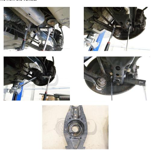
• With the OE LCA removed you can see the 4 holes in the arm that we are going to add the rivnut threads in to. For the UK kits we are using M8 rivnuts and the 4 holes need drilling out slightly to allow the rivnuts to mount in. Ideally an 11mm drill bit is needed.
